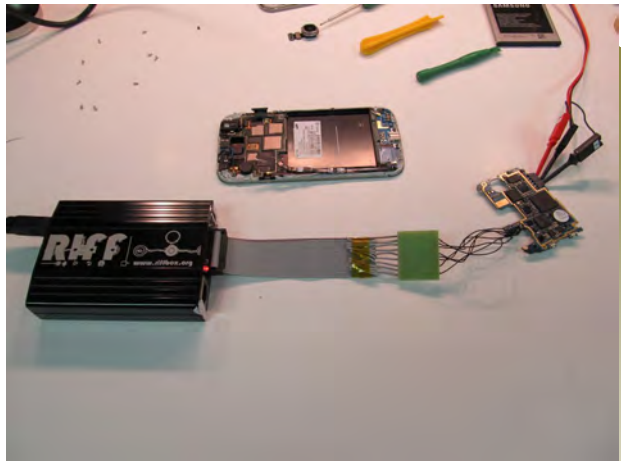
JTAG hardware hooked into a cell phone circuit board
