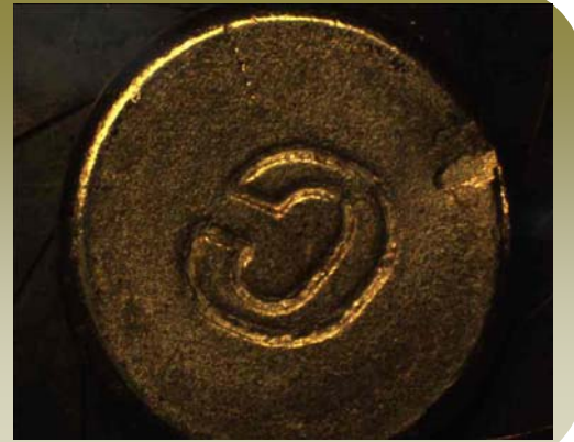
Firing pin indentation on the misfired cartridge.
