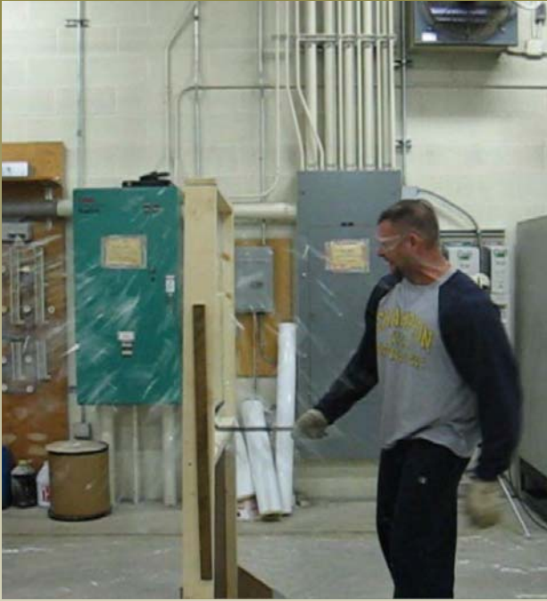
Green studying how broken glass particles transfer to clothing.
